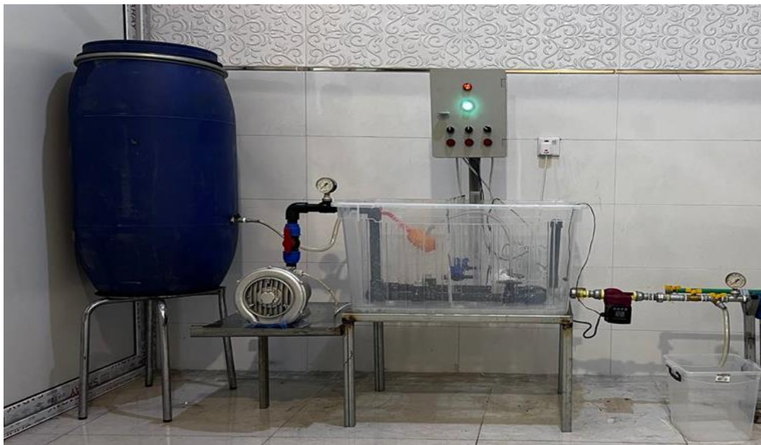
Figure 3: Anoxic Sequencing Batch Biofilm Reactor (ASBBR) Lab Scale Plant
