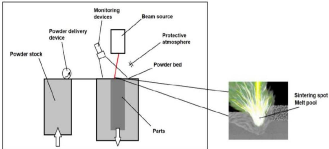
**Fig 2: Schematic representation of DMLS process**
