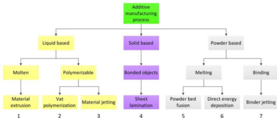
Fig 1: Classification of various Additive Manufacturing process
