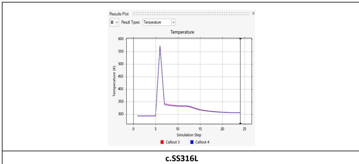
**Fig 7: Representing Temperature variance for 3 Materials in Rank-1position of part**
