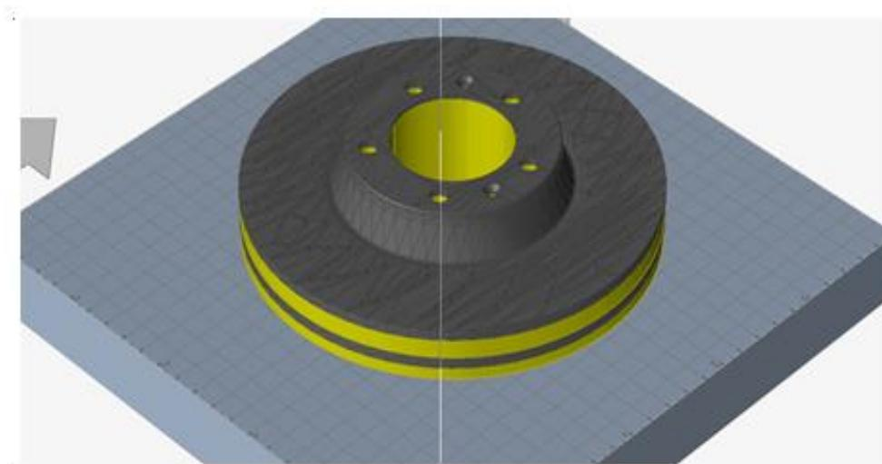
**Fig 4: Representation and position of the part on the build platform**
